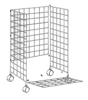
Using large plastic clips, attach one large grid (A) to the back grid (B), then attach the other large grid (A) to the other side of grid (B). Attach center grid (C) to bottom.
